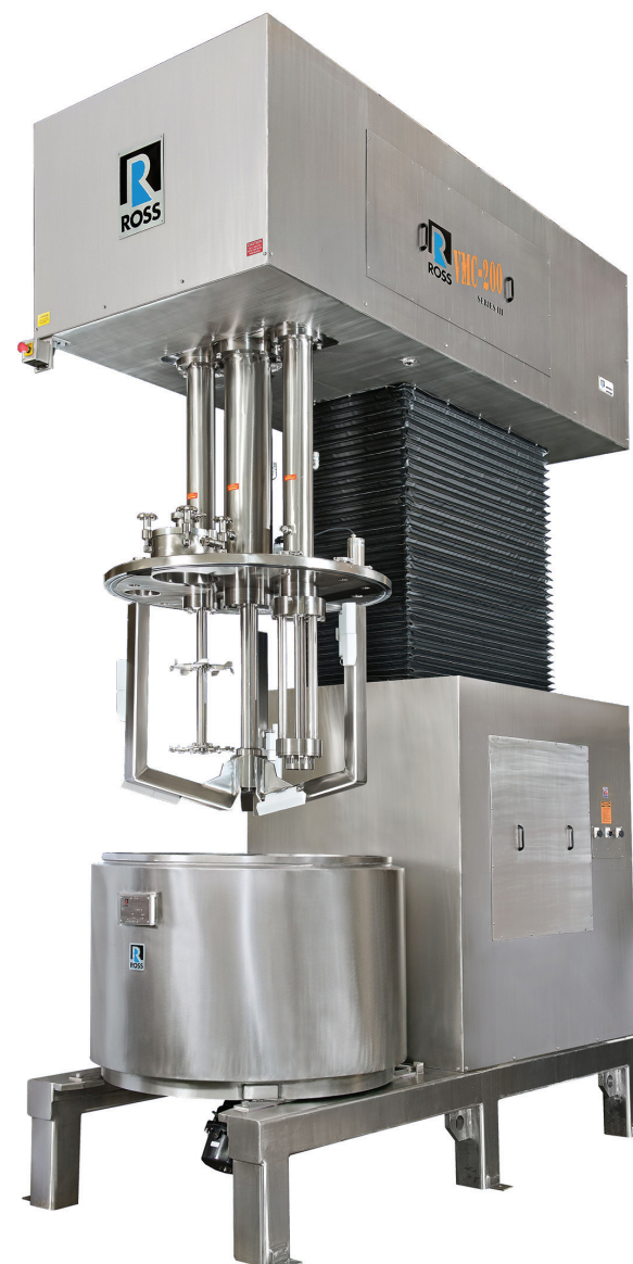
Figure 1. Multishaft mixer equipped with three independently driven agitators: three-wing anchor, high-speed disperser and high-shear rotor/stator mixer. This configuration is well-suited for medium- to high-viscosity applications such as slurries, pastes and suspensions up to several hundred thousand centipoise (cP).
